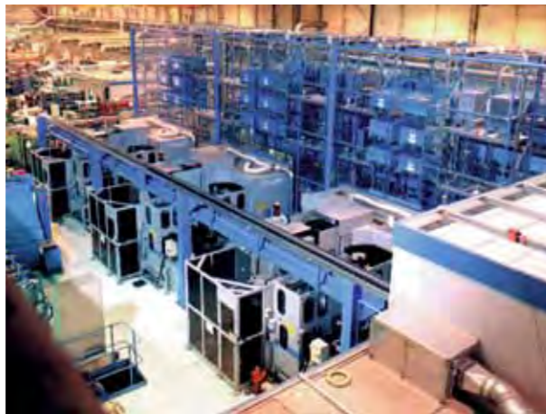
Automated Central Tool Storage, CTS, with Tool Gantry enables location of all spare tools in a central magazine and automates tool change to MC magazines from Central Tool Storage.
